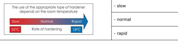
The type of used hardener affects coating drying time and depends on room temperature and the preference of the painter. Proper selection of the type of hardener ensures appropriate structure and appearance of coating.
