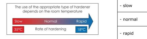
The type of used hardener affects coating drying time and depends on room temperature and the preference of the painter. Proper selection of the type of hardener ensures appropriate structure and appearance of coating.
